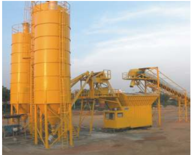
18 year old M1 Batching plant working at L&T Project site
