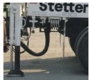
Outriggers at the rear to provide support
