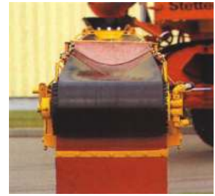
110° belt trough angle for reliable and clean material conveyance
