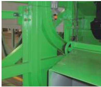
Double skip rail track
